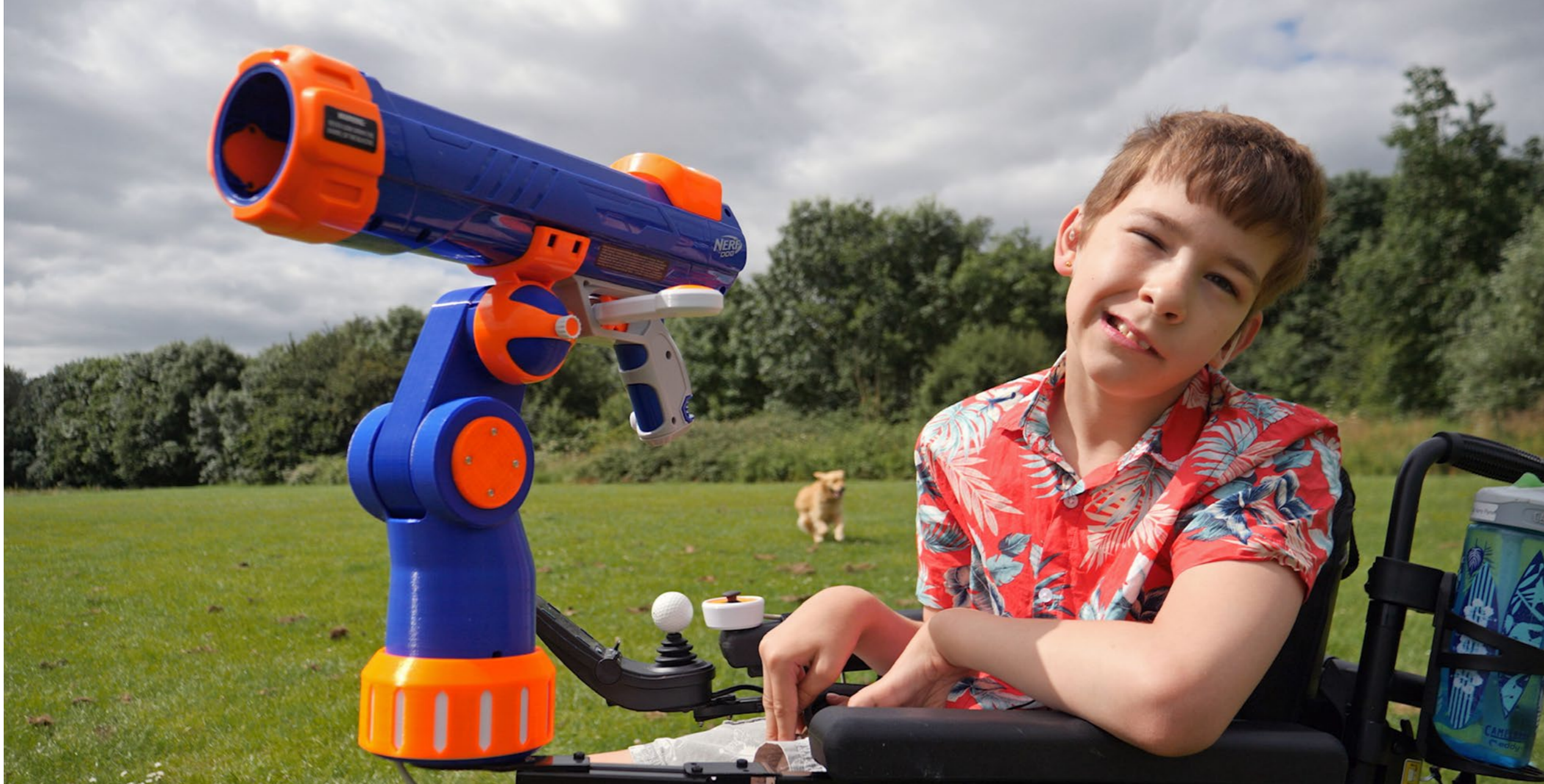
Ball Launcher - Enabling Harry to throw a ball for golden retriever Addi was achieved by CIC combining a Nerf ball launcher and our very own 3D printed joystick controlled arm.
